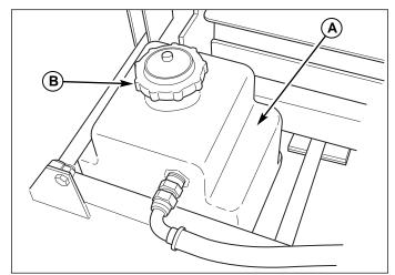
Figure 14. Hydraulic Oil Reservoir
